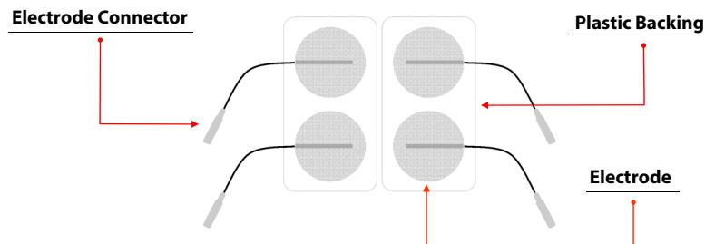
**Step 2** Insert lead wire pin connectors into electrode connectors as shown below. **RED** lead wire connectors on one side and **BLACK** lead wire connectors on the other side.
